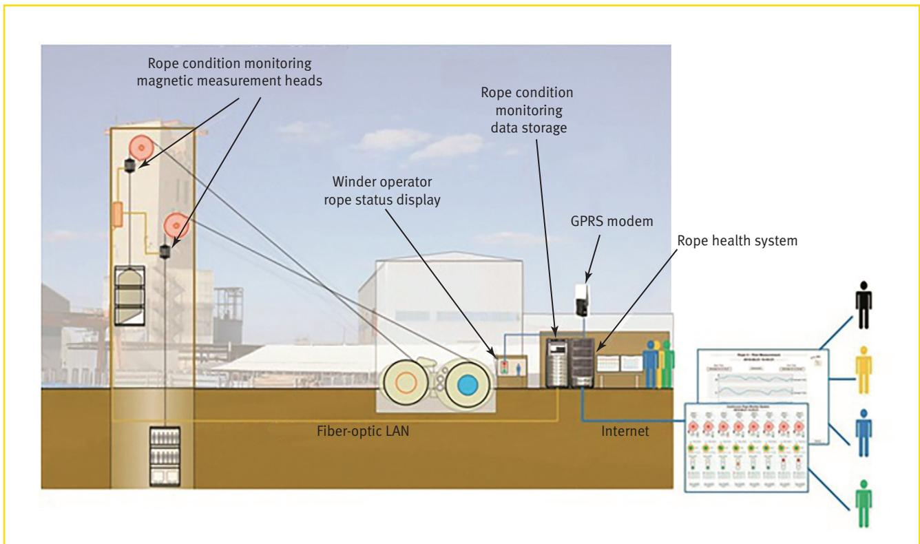
**Figure 4.** The rope monitoring station is located in the mine control room, where information on the ropes' conditions is streamed continuously.
