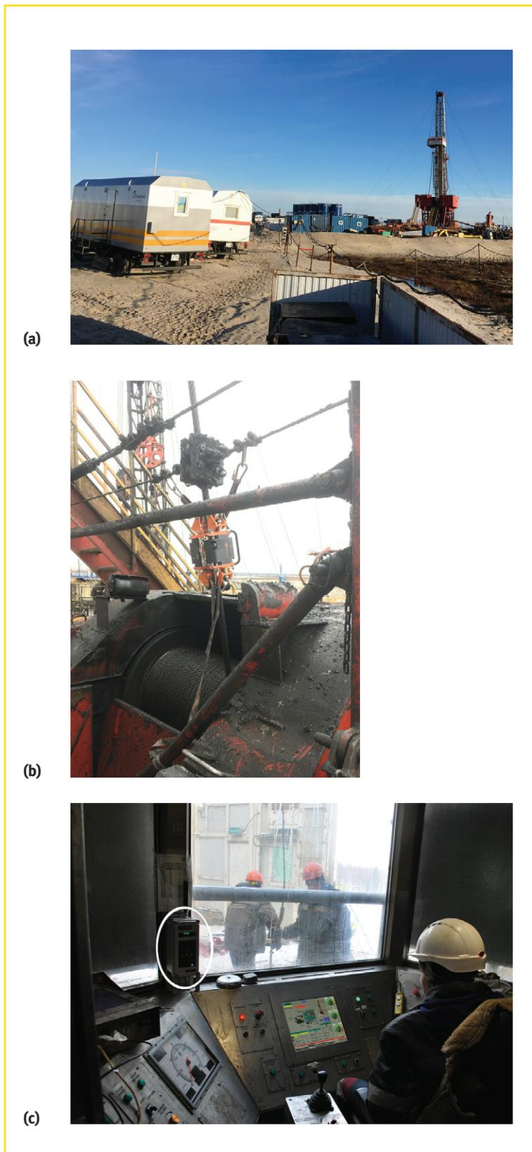
**Figure 3.** A typical drilling rig installation: (a) drilling rig on job site; (b) the magnetic head installed above the drum; (c) the control and display unit in the operator's cabin (circled).
