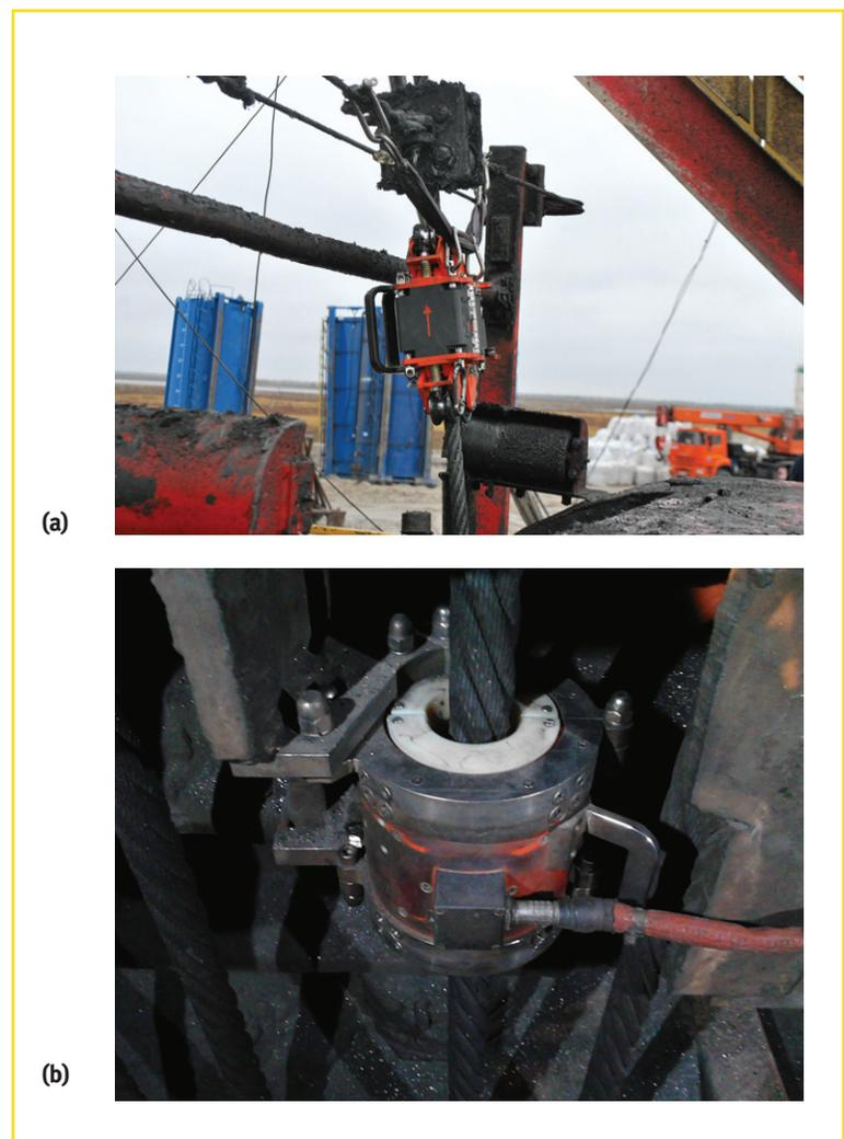
**Figure 2. Two designs of a magnetic head for an automated condition monitoring system: (a) design for periodic monitoring of a drilling rig calf line; (b) design for more permanent installations, such as hot-metal crane ropes.**
